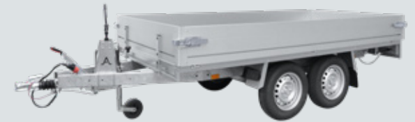
KLT tandem braked with hydraulic hand pump
