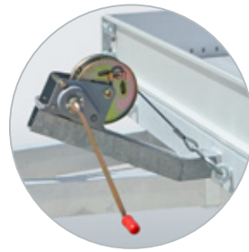
An adjustable winch support for left- and righthand use
