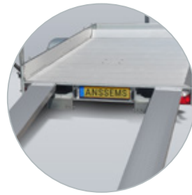
Aluminium ramps in integrated ramp holders
