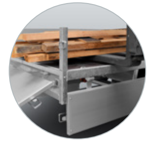
Panels that rotate below the floor. Damage-free loading and unloading.
