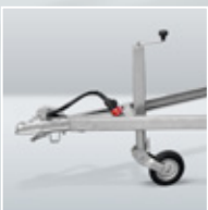
Unbraked BSX version: A-frame of U-profile (length 135 cm.)
