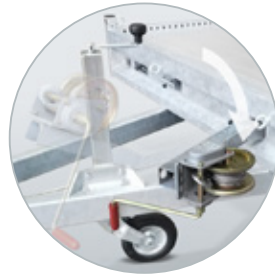
Accessorie: In length adjustable and rotatable winch
